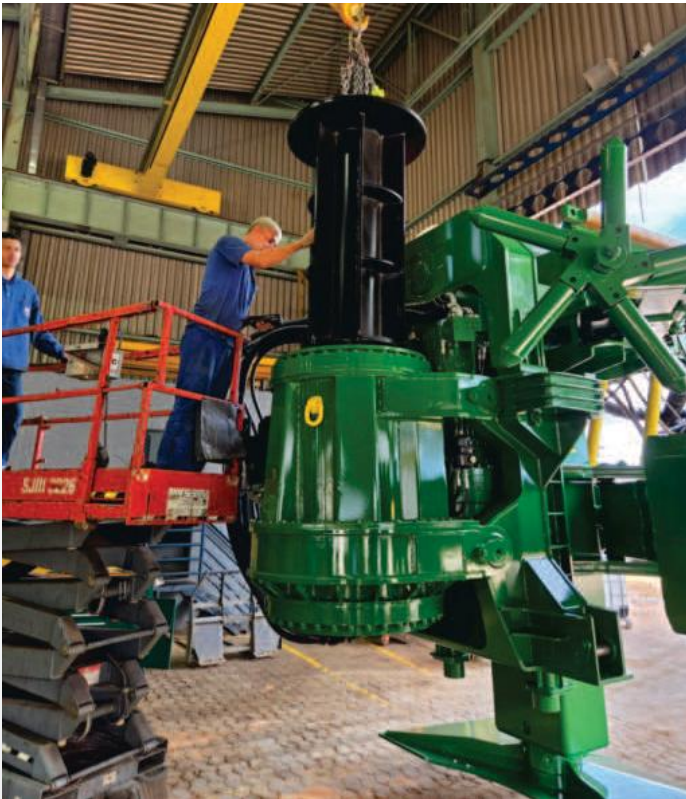
1- Adaptador para CFA e 2 - Roldana CFA 1 – CFA adapter and 2 – CFA sheave
