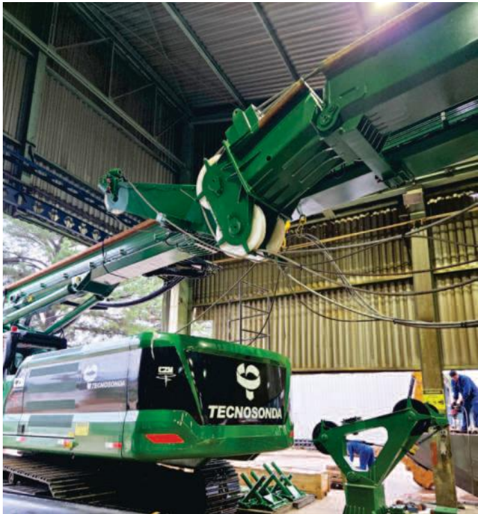
Torre com cabeça de CFA com dobra hidráulica Mast with CFA head and hydraulic folding
